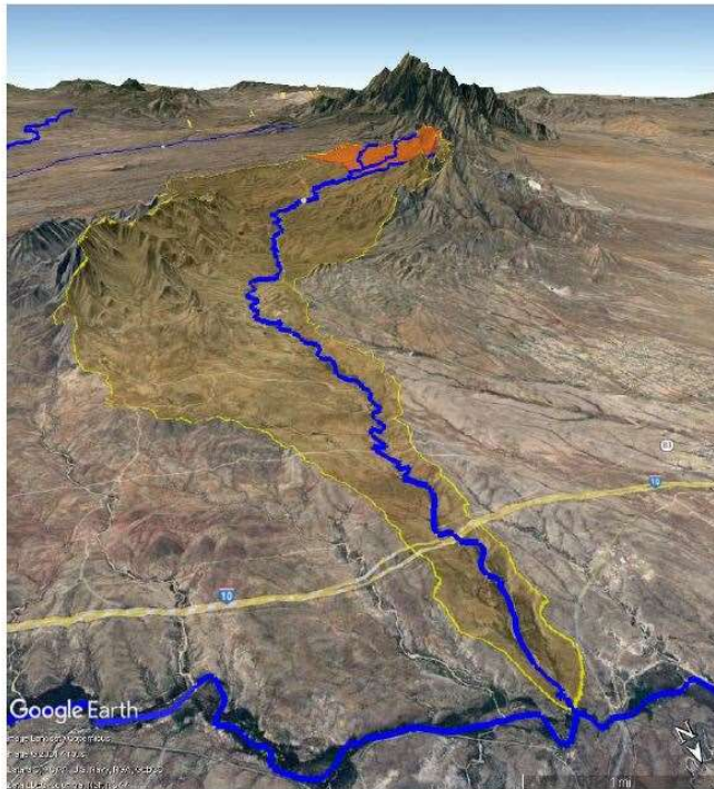
Watershed delineation by USGS StreamStats. 3D elevation not to scale.
