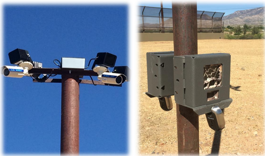
Figure 2. Structure surveillance system components: video camera with infra-red lights (left) with still camera (right) as backup documentation at the overpass and to capture wildlife use at the underpass
